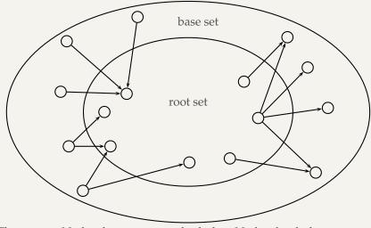
The root set Nodes that root set nodes link to Nodes that link to root set nodes The base set
